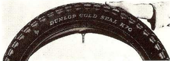
Fig. F13. Cover and tube assembled ready for refitting to the wheel
