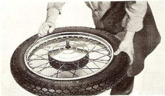
Fig. F11. Removing the first bead of the tyre—Lever inserted close to valve whilst bead is pressed into well on opposite side of wheel
