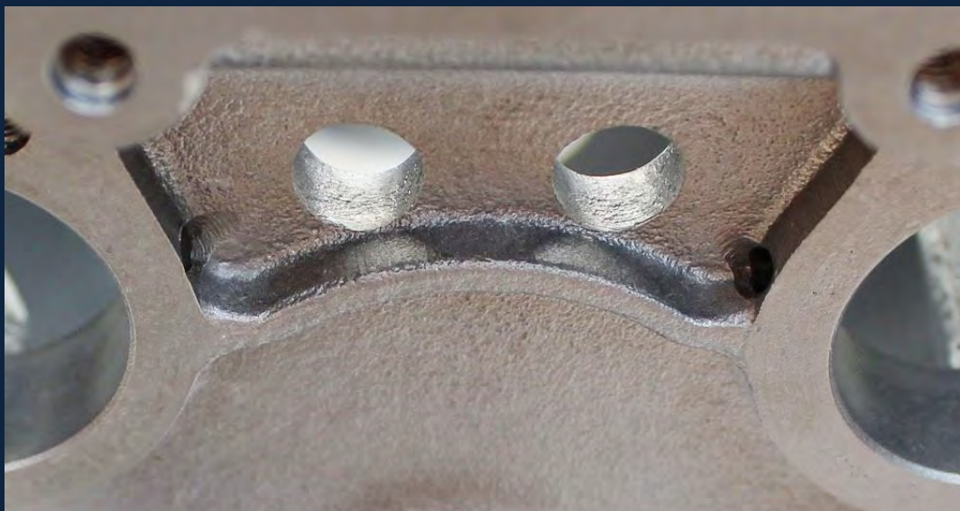
Detail of the Oil Weirs and Galleries as described above.
