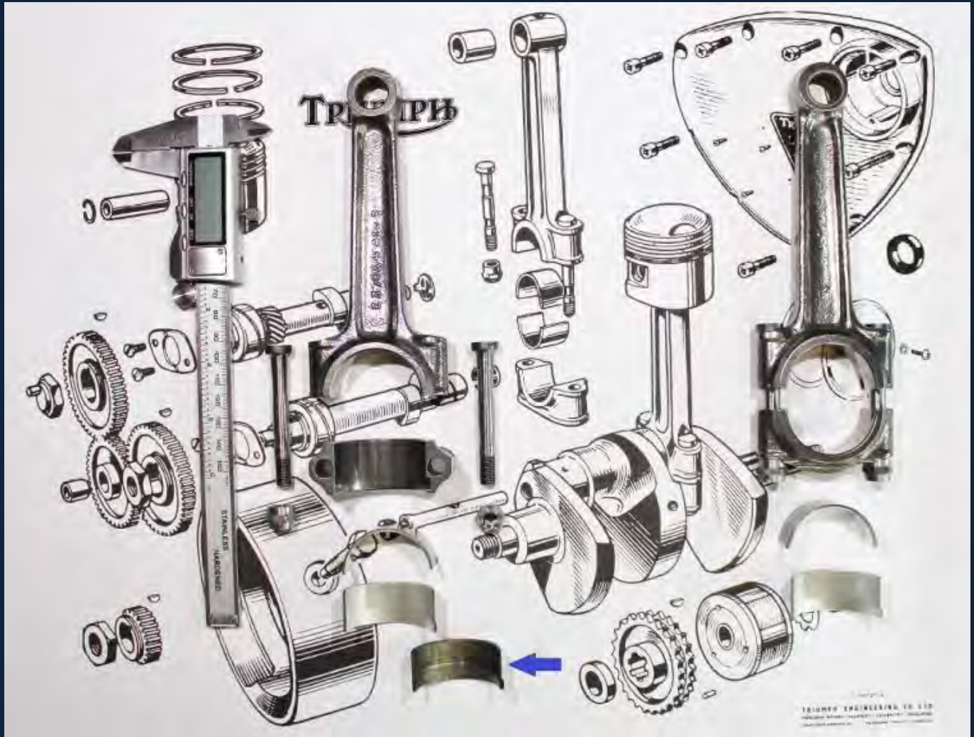
The Connecting Rods, Caps, Shell Bearings and Bolts.
