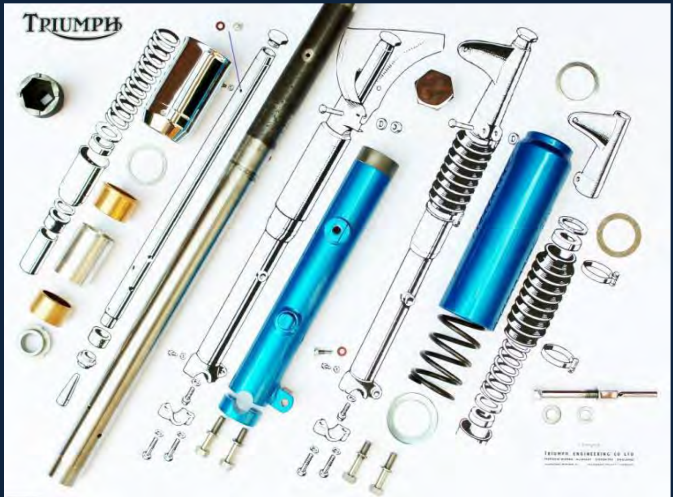
The Fork Parts Nacelle Type 1965-1966
