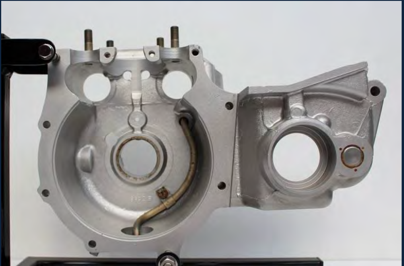
Crankcase Timing Side Internal View
