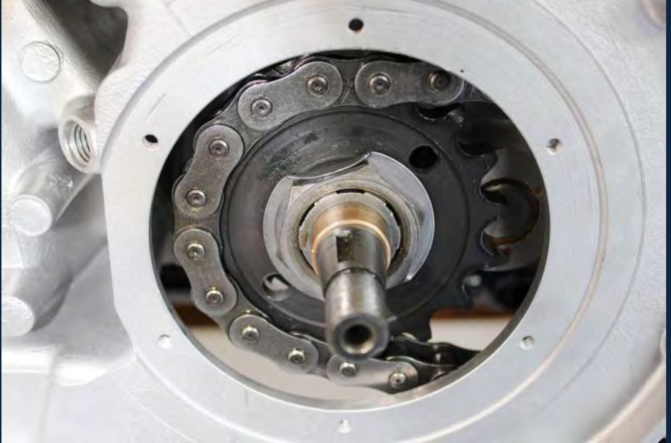
The Chain Fitted, Nut Tightened and Locked.
