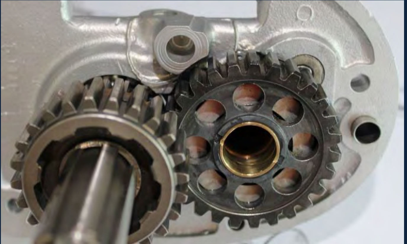
Mainshaft with First and Second Gears Fitted
