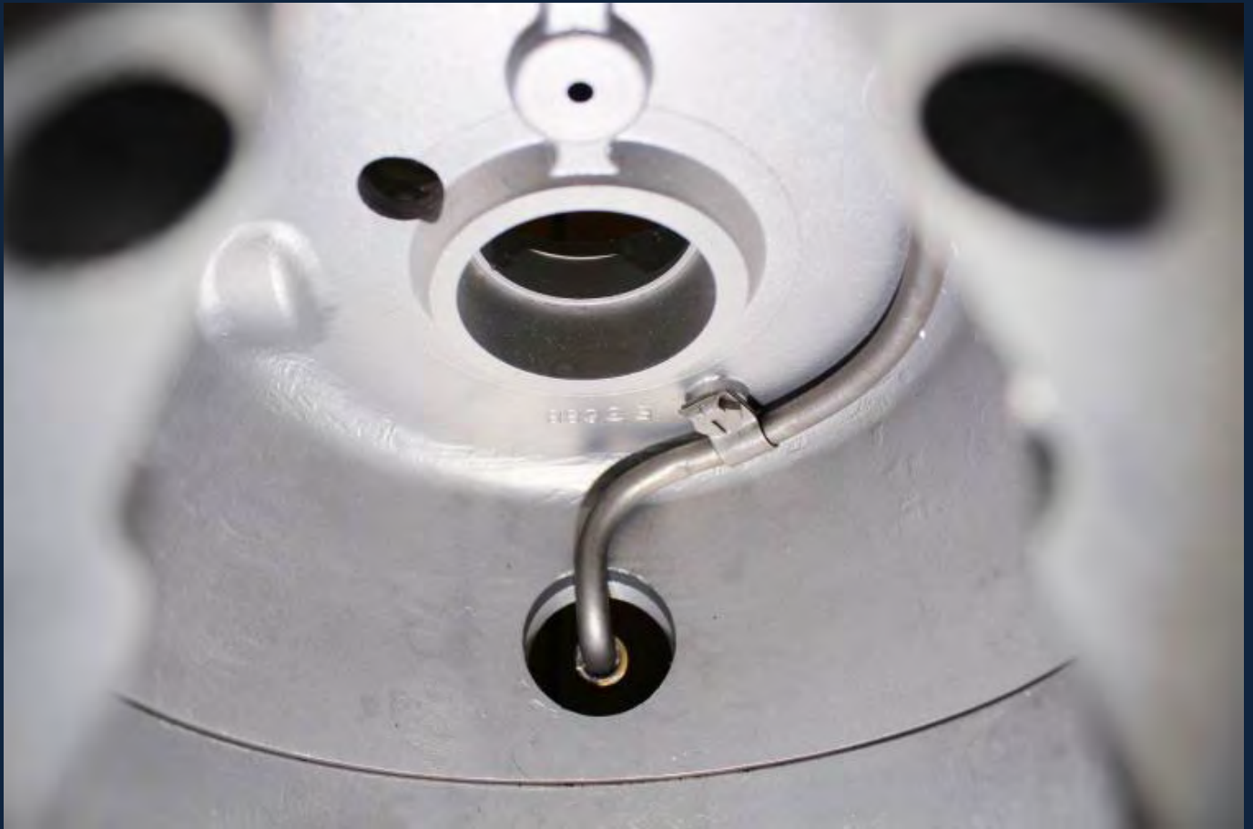
The Timing Side and Oil Pick Up Tube
