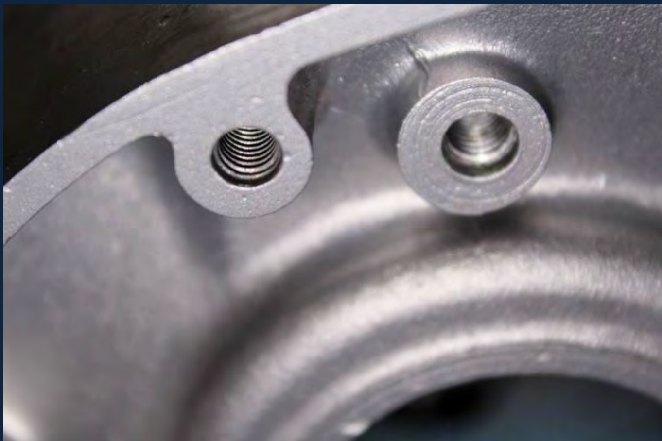
One of the numerous \frac{1}{4} BSF Threaded Holes, here in good condition.
