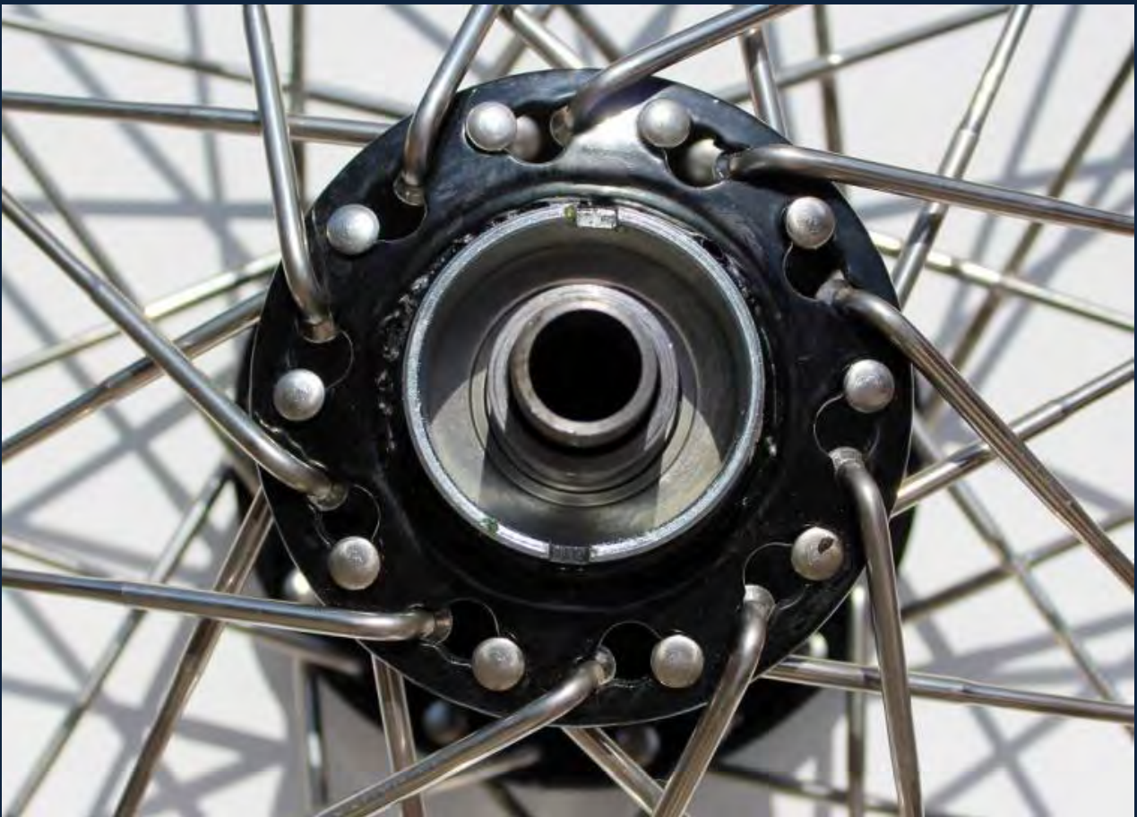
The (Later) Complete Hub showing The Speedo Drive Sleeve
