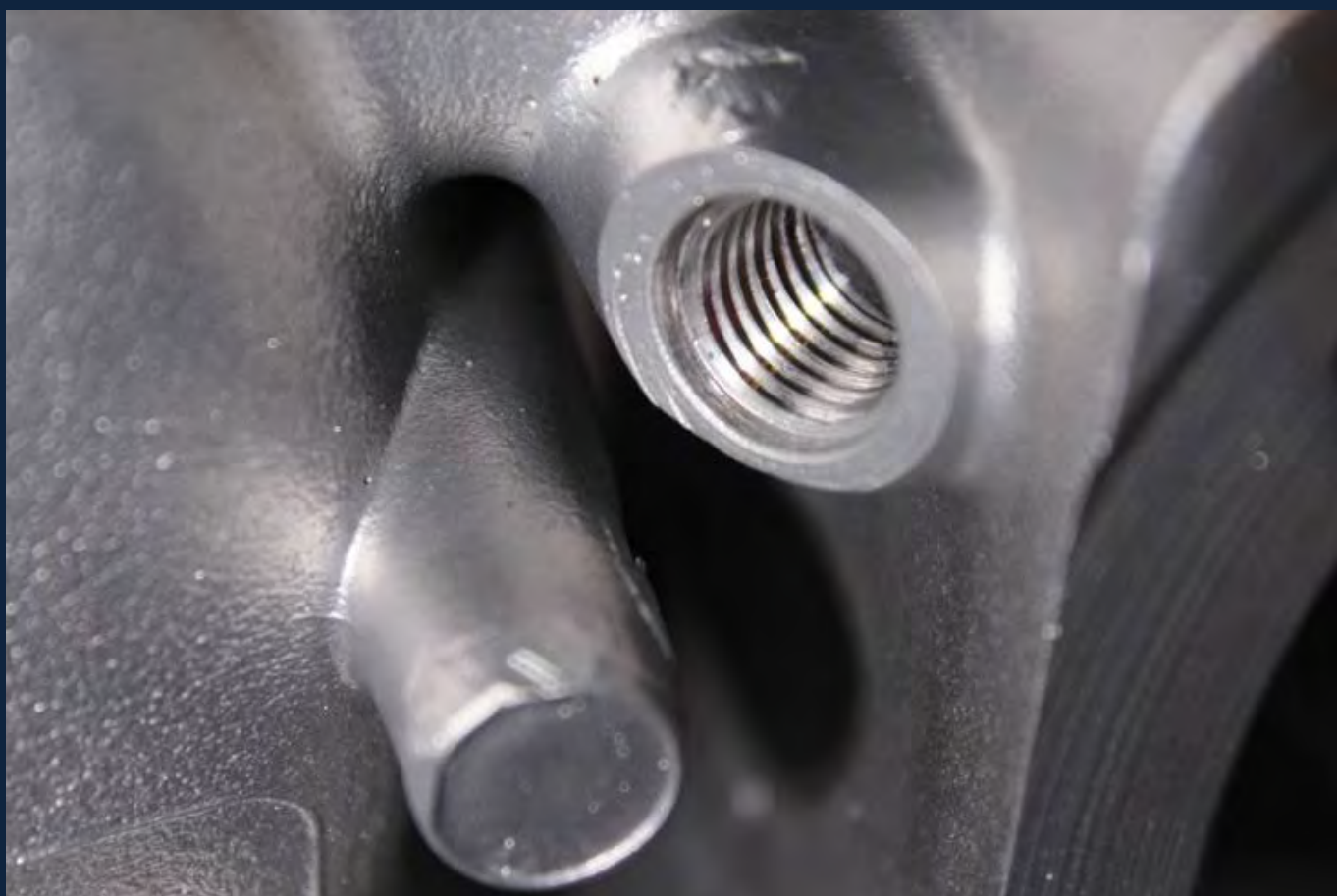
The Alternator Cable Exit. \frac{1}{2} in BSF after Tapping and Cleaning. Also, \frac{1}{2} in BSF the TDC Plug, Gearbox Drain and Rev Counter.
