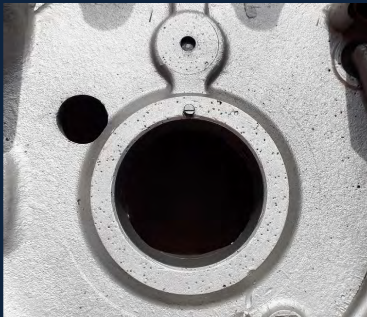
The Raised Pip on the early Crankcase
