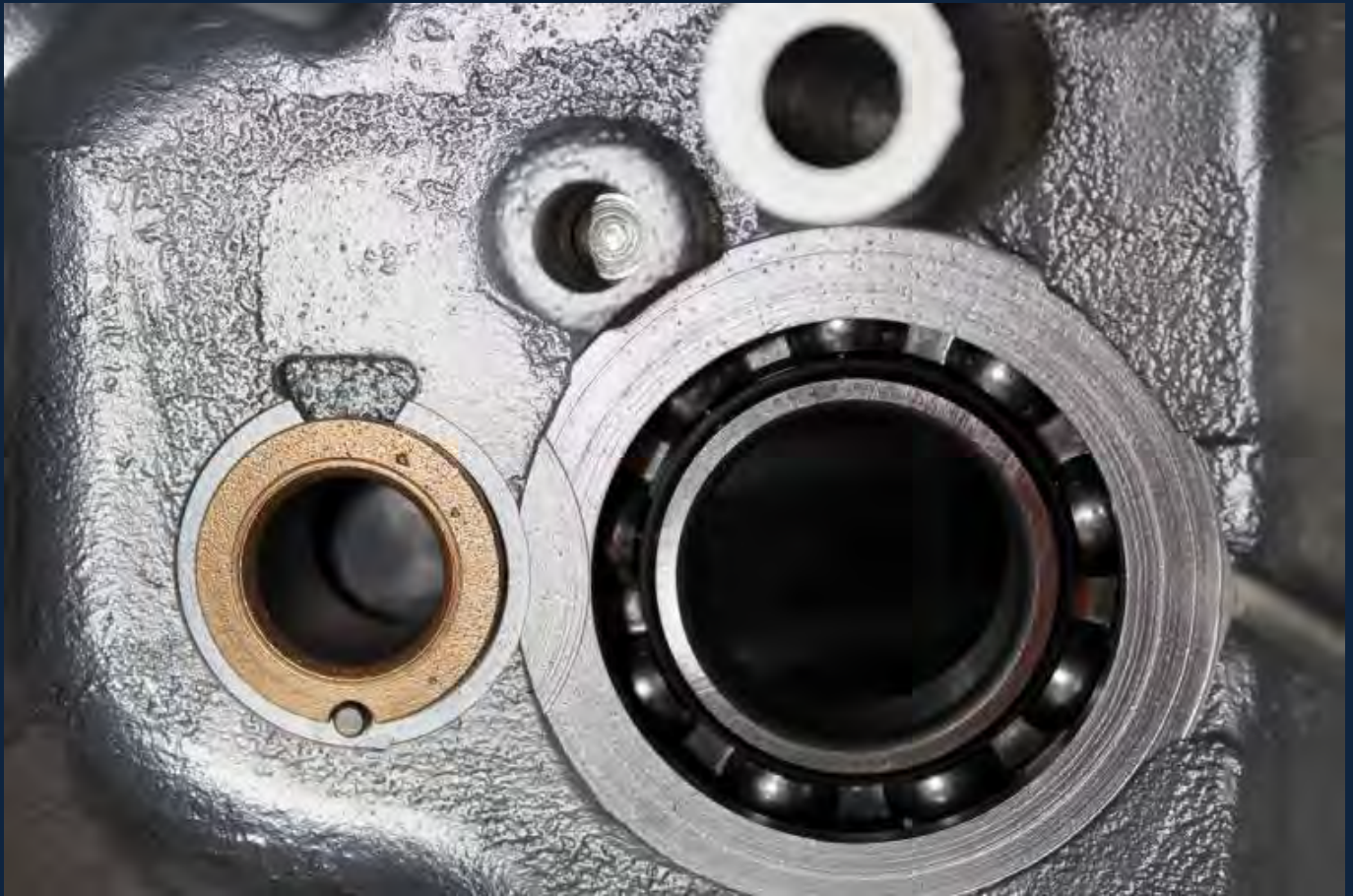
Detail of the Gearbox Bearing and Layshaft Bush
