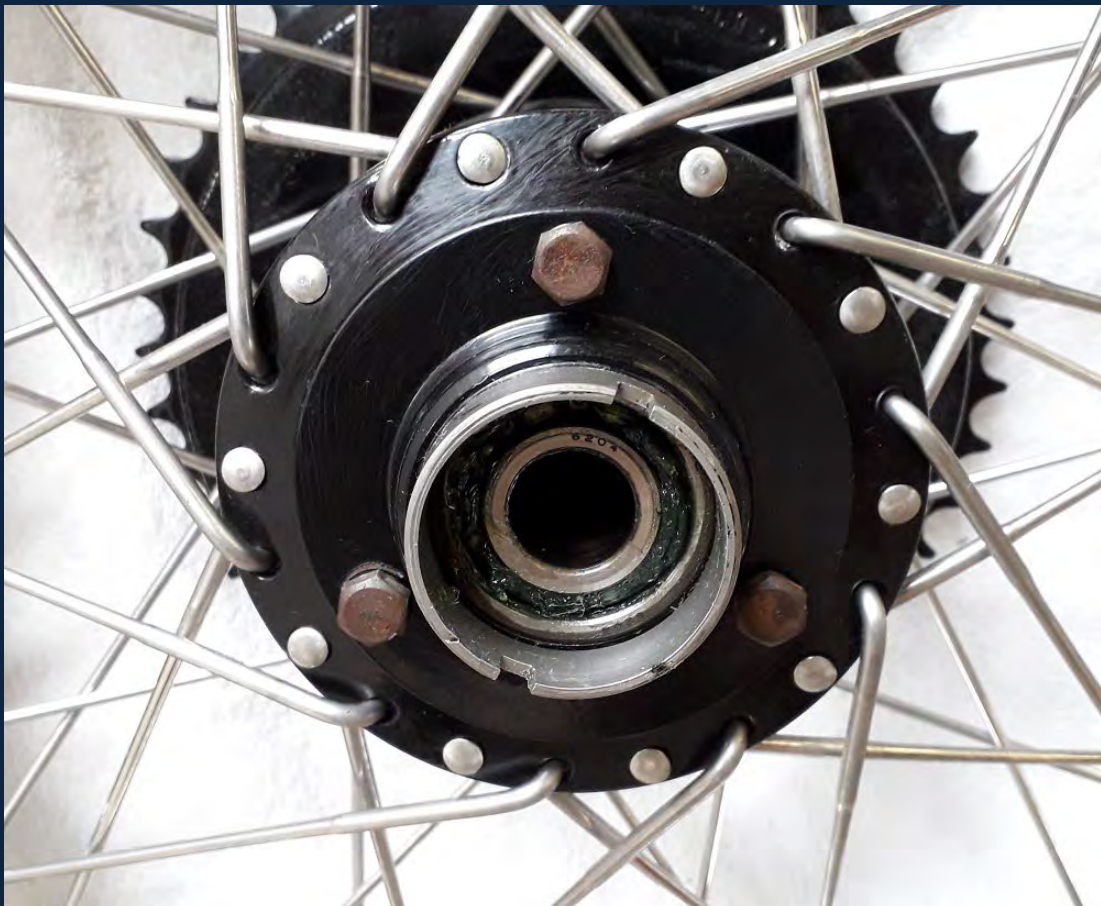
Early hubs as above, have a bolted-on drive sleeve and a different spoke flange.
