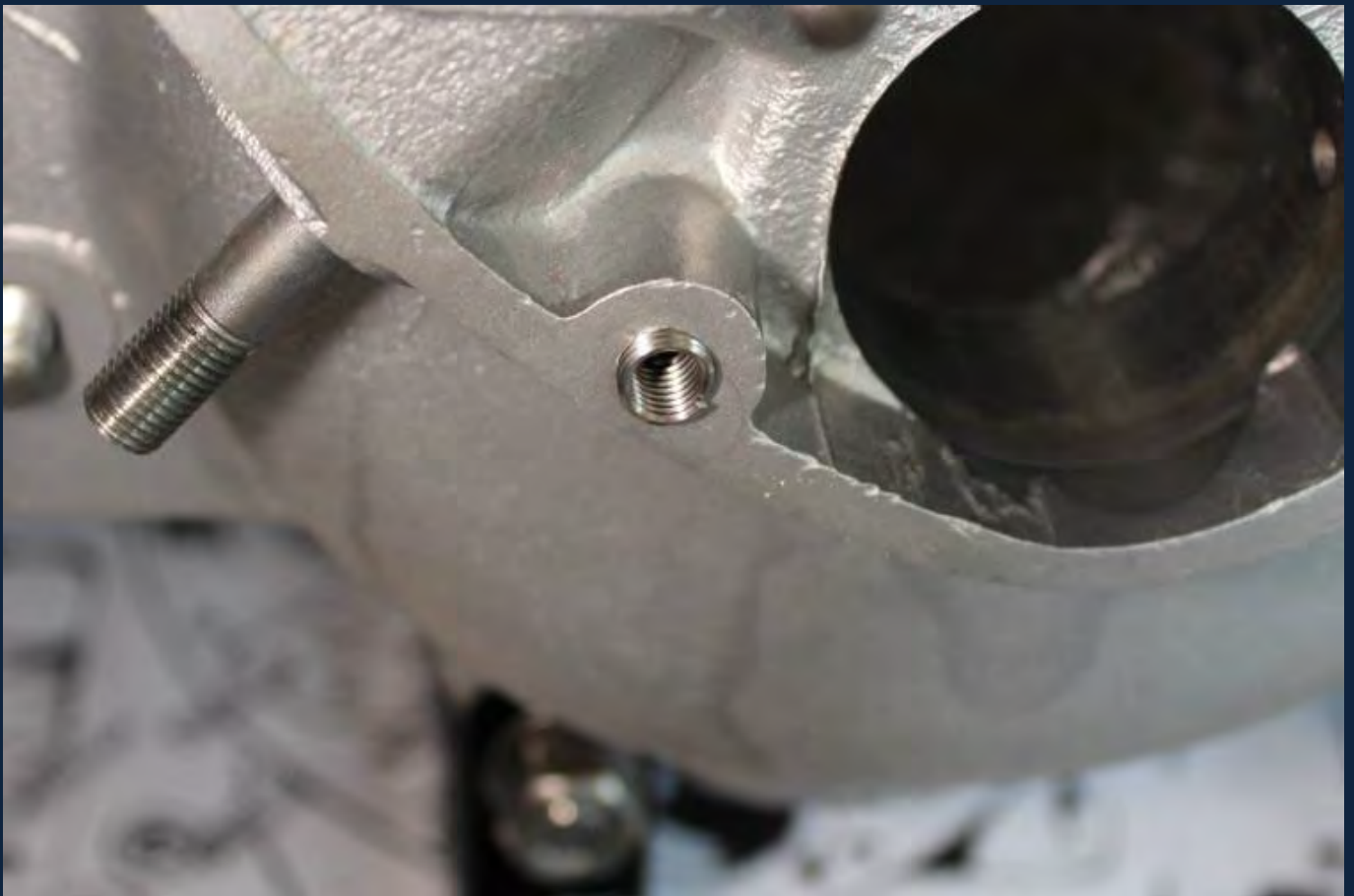
The Helicoil partially inserted into the cleaned hole.
