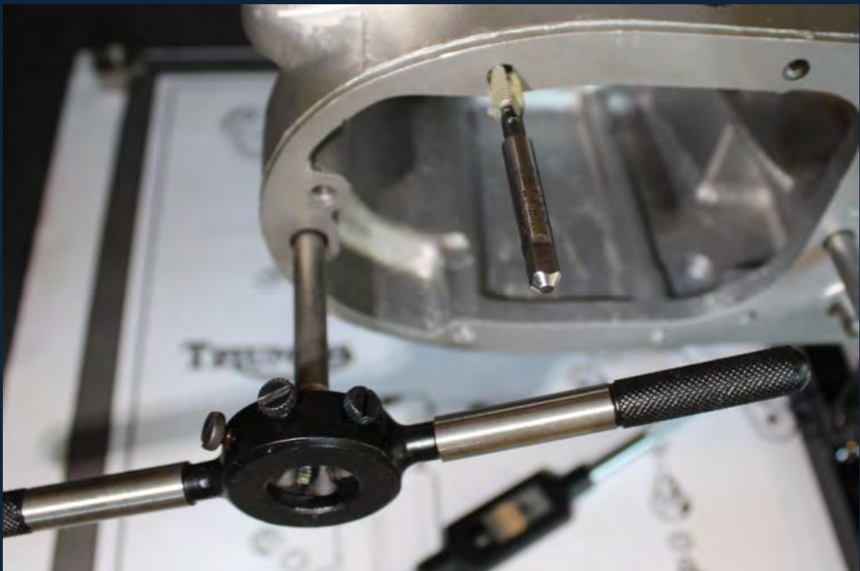
Using Taps and Dies to Cut and Clean the Threads.
