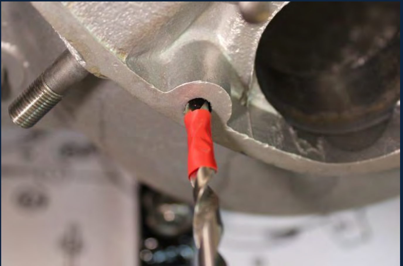
Using the drill size recommended the damaged hole is cleared, tape the drill to set the required depth.
