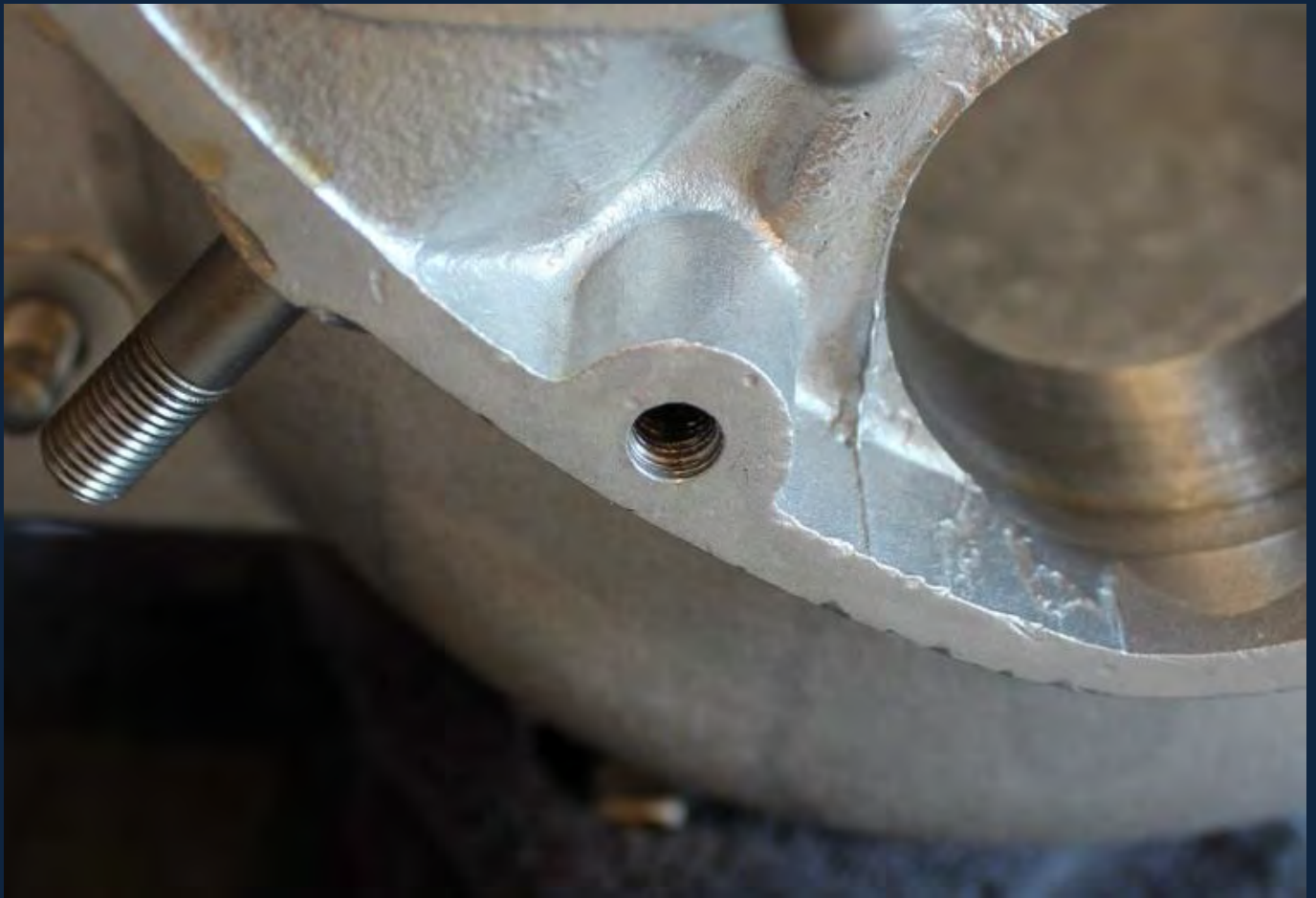
A Damaged Thread... A Helicoil will be needed.
