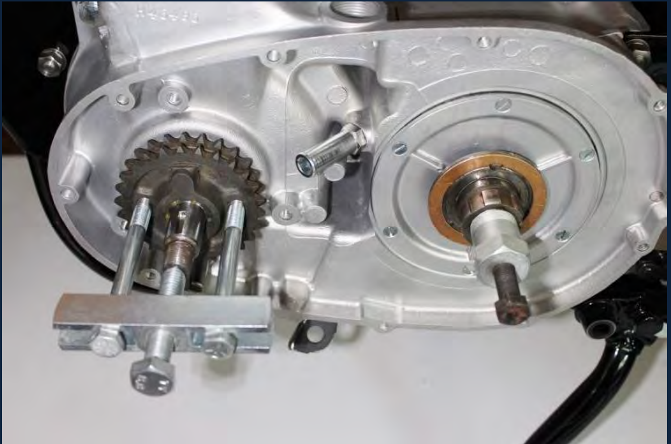
Showing the Pullers to remove the Sprocket and the Hub (The Puller on the left is also suitable for removing the gearbox sprocket)
