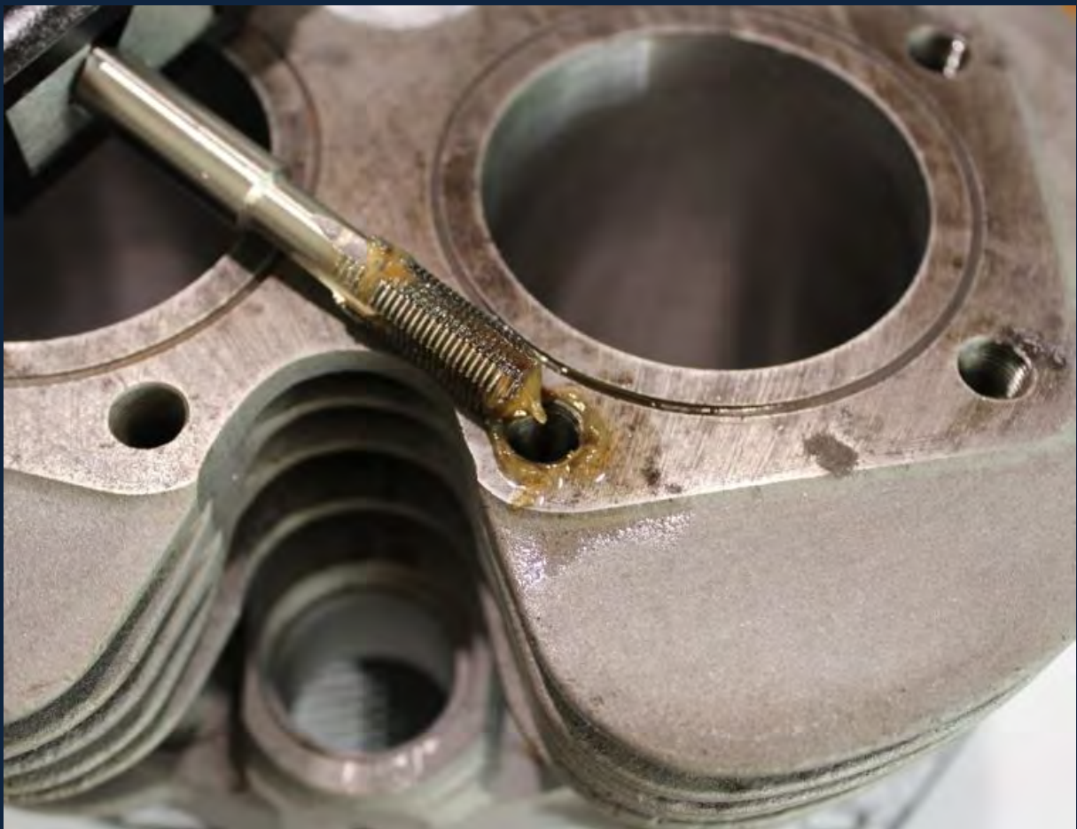
Residual blasting media and swarf sticking to the grease
