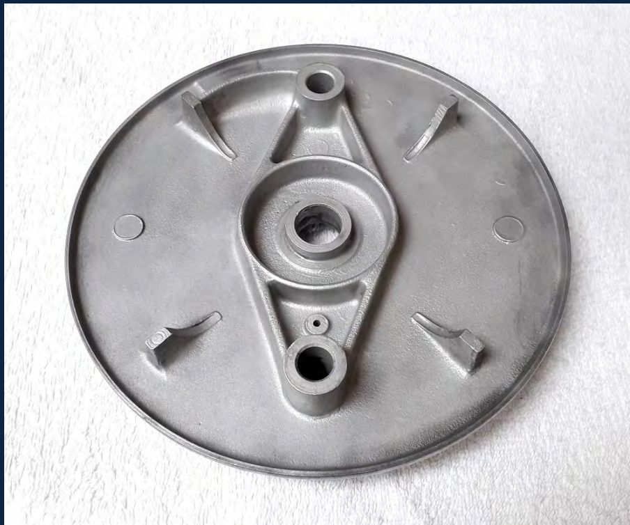
Early W1301 brake plate showing the additional support lugs not usually seen after 1960. There are several types of 7 in brake plate fitted across the range including the sought-after twin leading shoe type. Some Daytona models use the 8in Brake and Hub From the larger B Range Machines.
