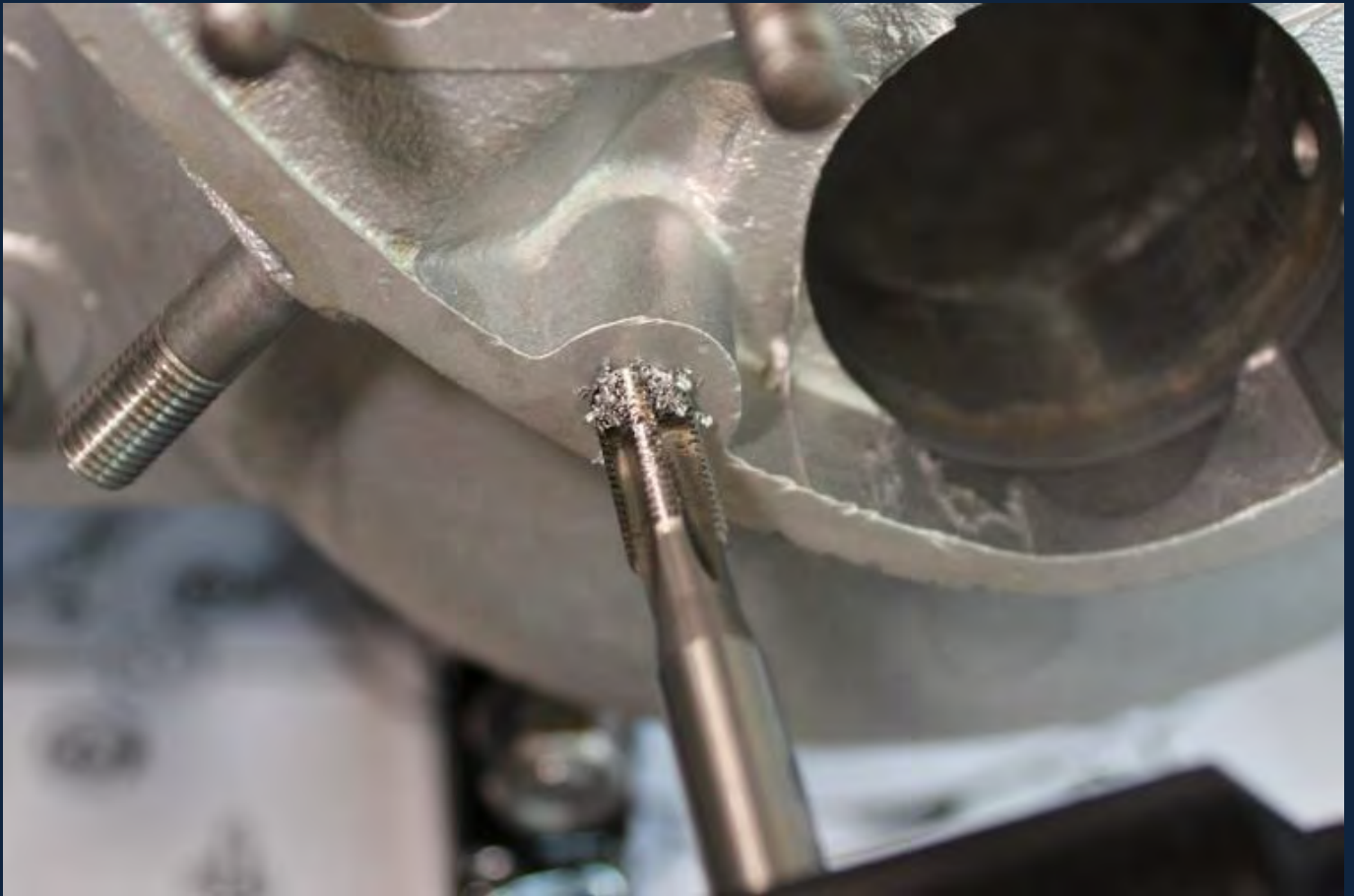
Using the Tap from the Helicoil kit to Tap the hole.
