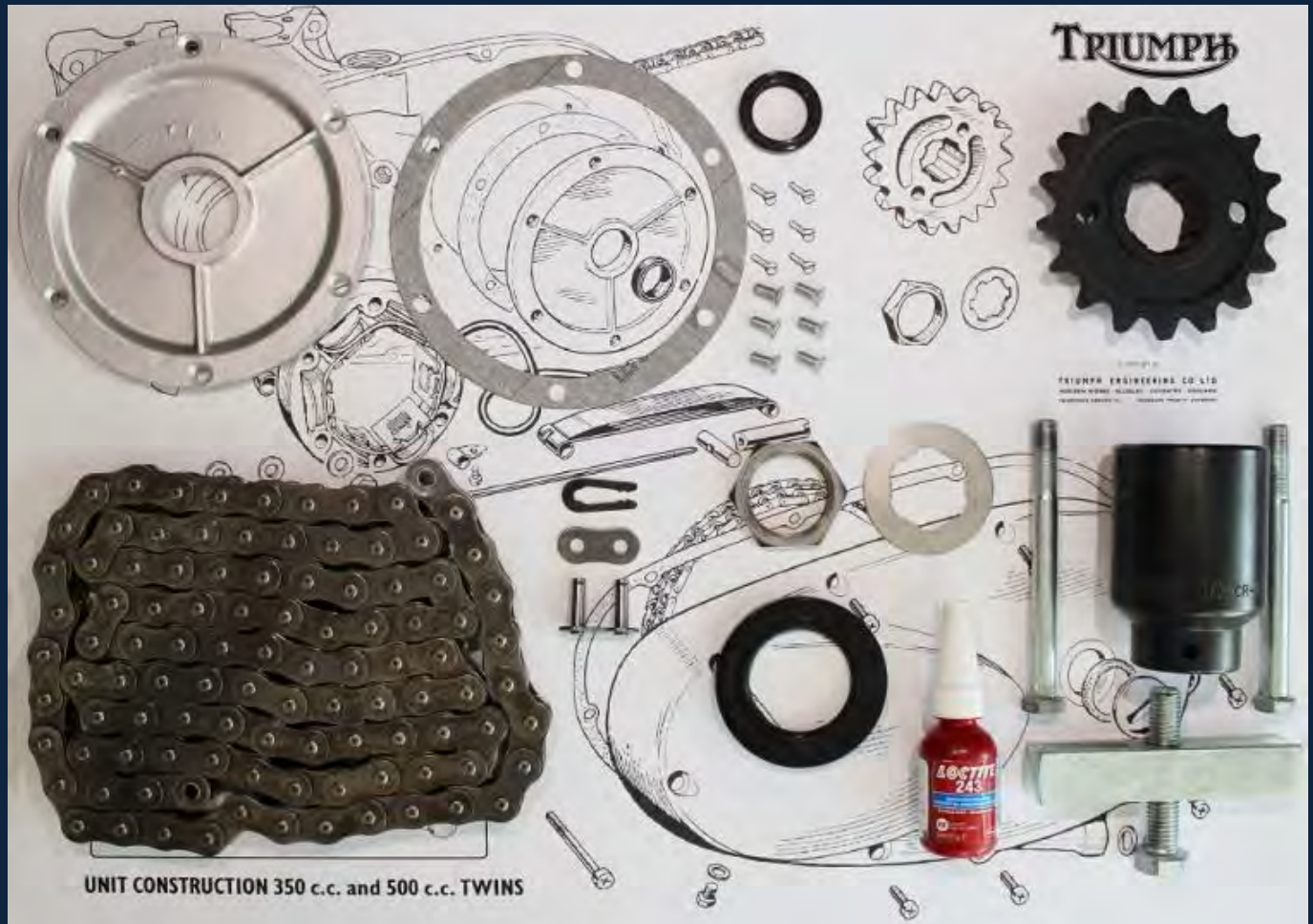
The gearbox sprocket, chain, seals, parts and tools.
