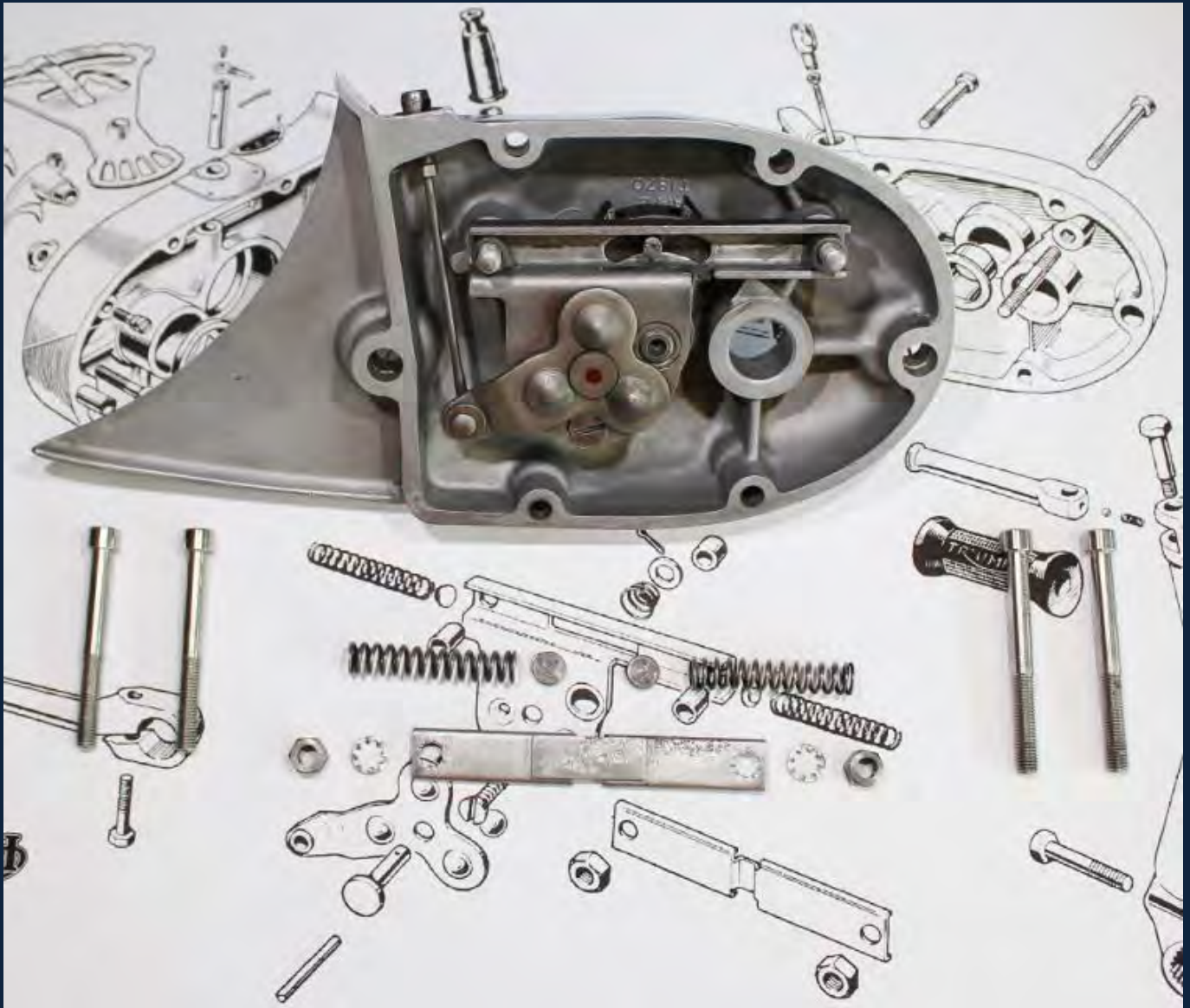
Assembly of the gear change mechanism.
