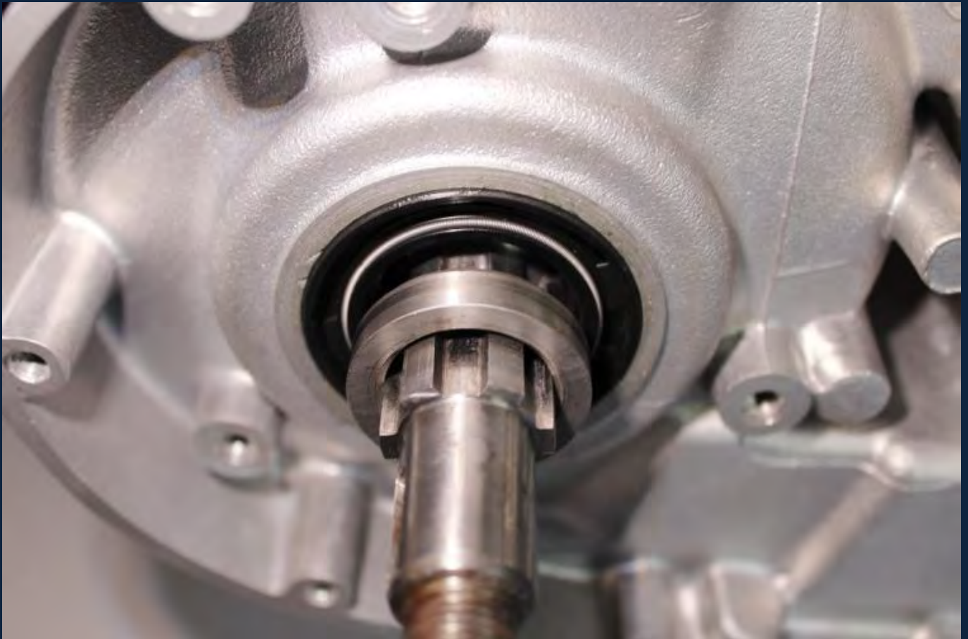
The Crankshaft Oil Seal and Ground Spacer.
