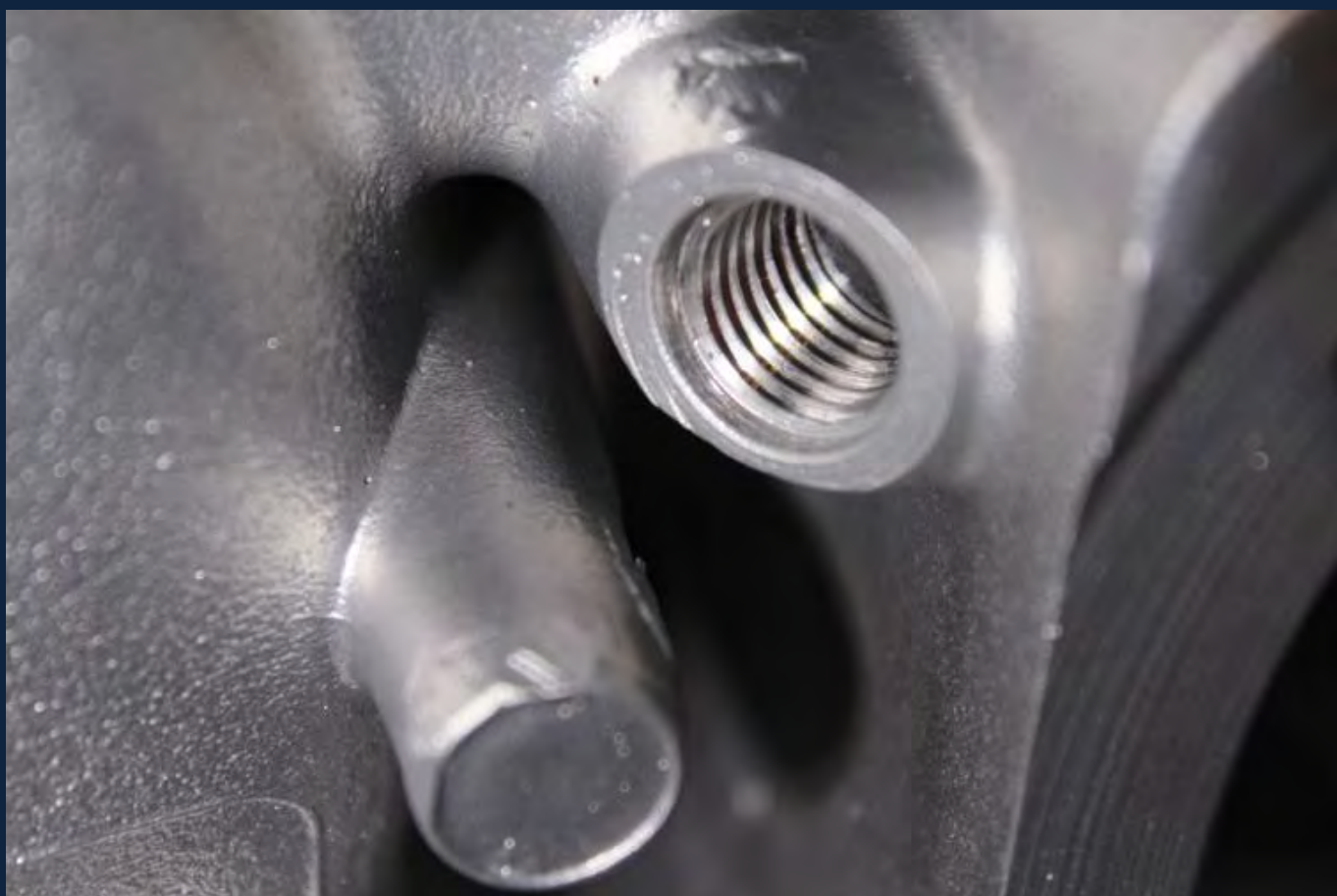
The alternator cable exit. \frac{1}{2} in BSF after tapping and cleaning, also \frac{1}{2} in BSF the TDC plug, gearbox drain point and rev counter location.
