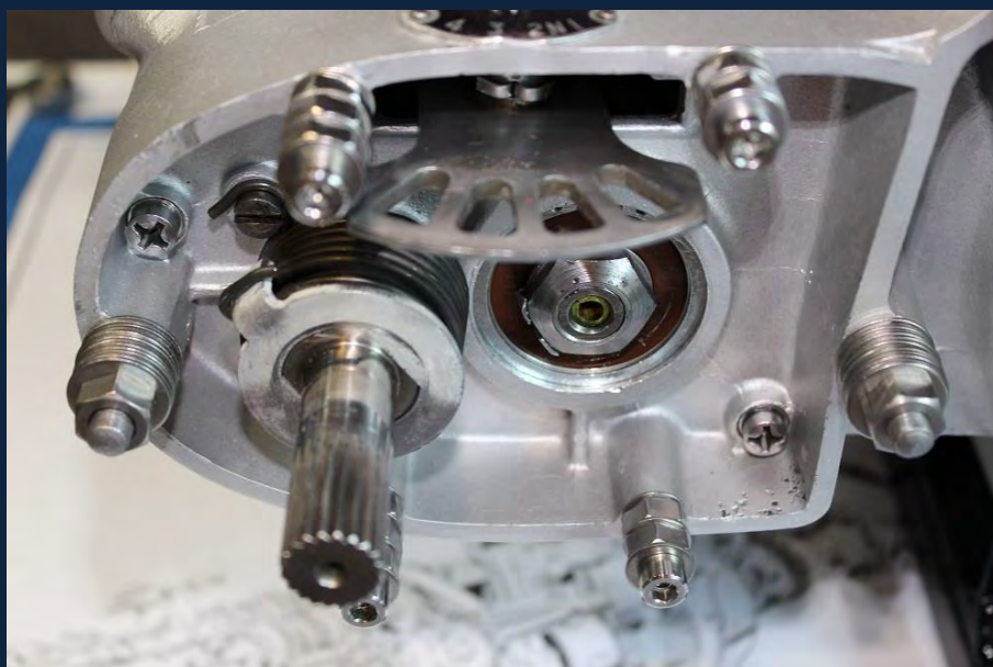
Holding the inner cover in place while the sealant sets, alternatively fit the outer cover even if only temporarily.
