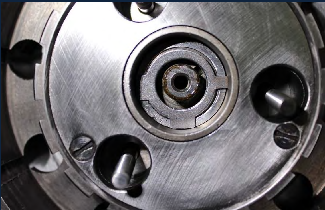
Here showing how the lock washer locates in the shock absorber hub. When the nut is tightened it distorts slightly allowing one of the two larger ears to be bent forward against a 'flat' of the nut.
