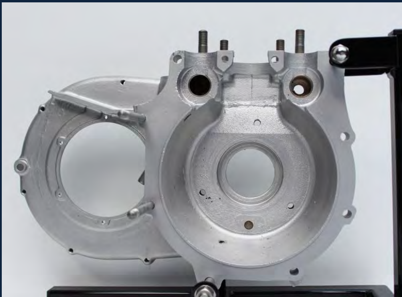
Crankcase Drive Side Internal View.
