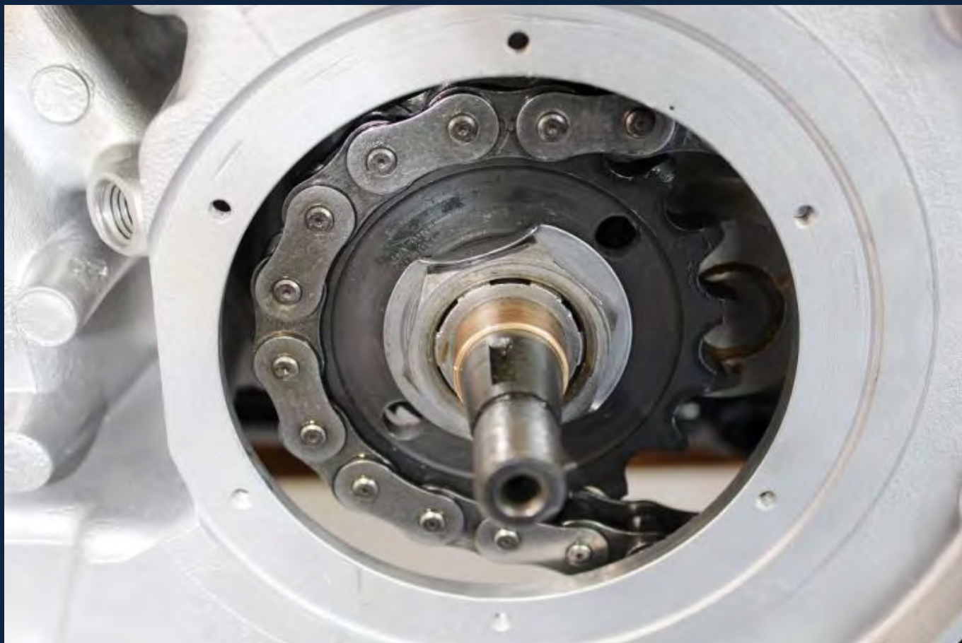
The chain fitted, nut tightened and locked.
