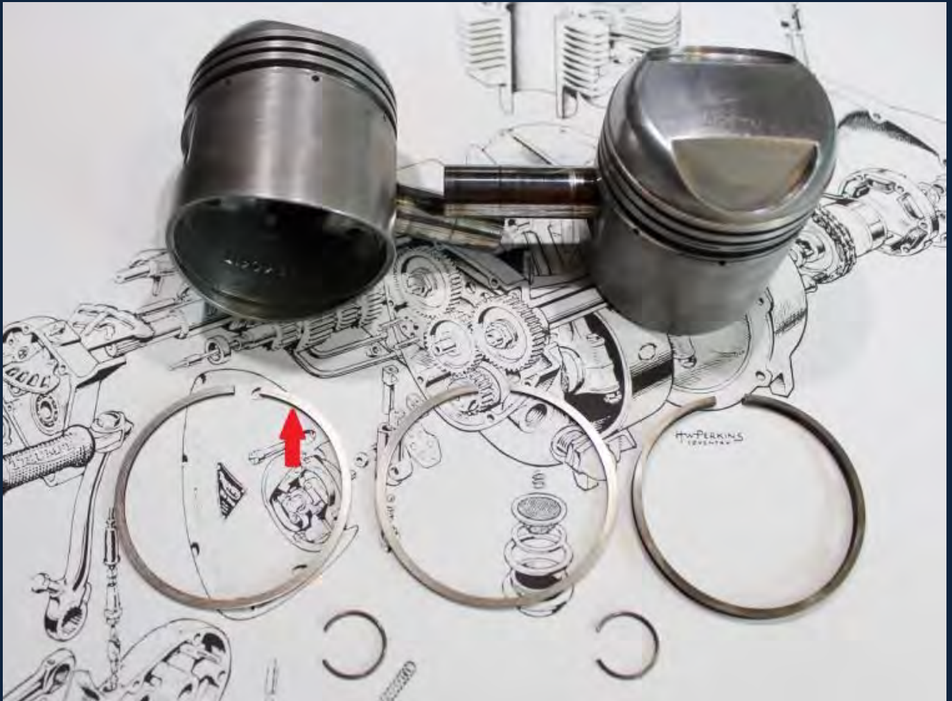
The Pistons, Pins, Rings and Circlips.
