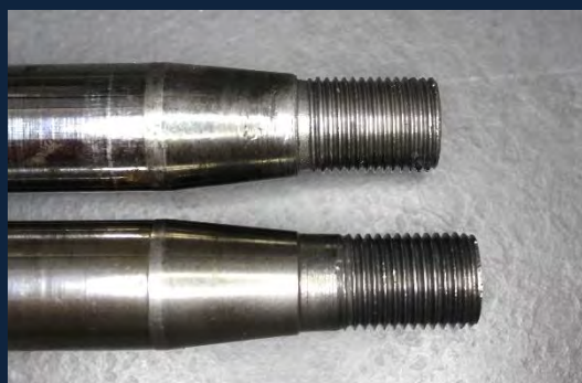
For illustration an early Mainshaft (to 1968) top, later below.
