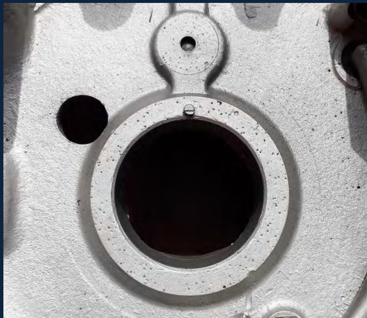
The raised pip on the early crankcase.
