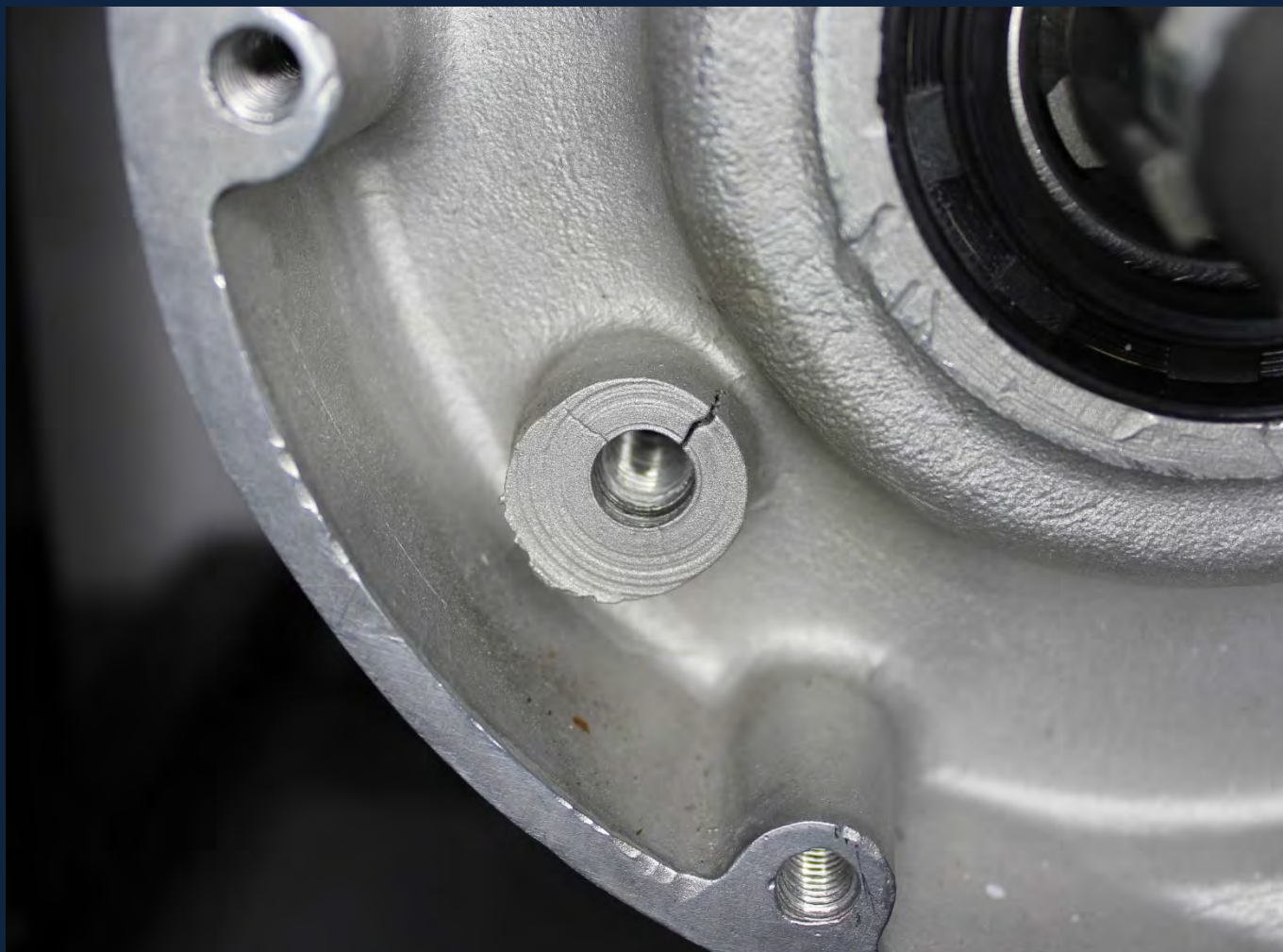
A cracked stud location, quite common; this will need specialist welding.
