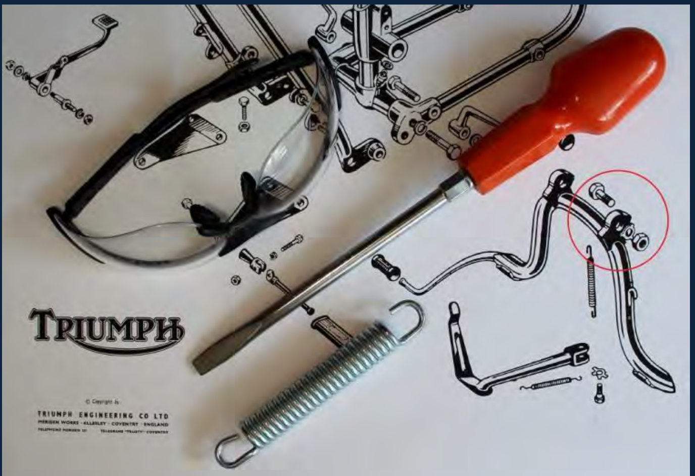
Fitting the Main Stand and Spring.
