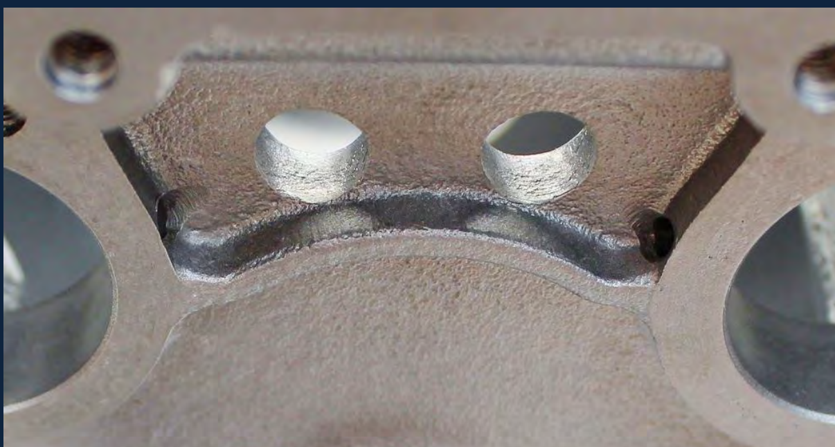
Detail of the oil weirs and galleries as described above.
