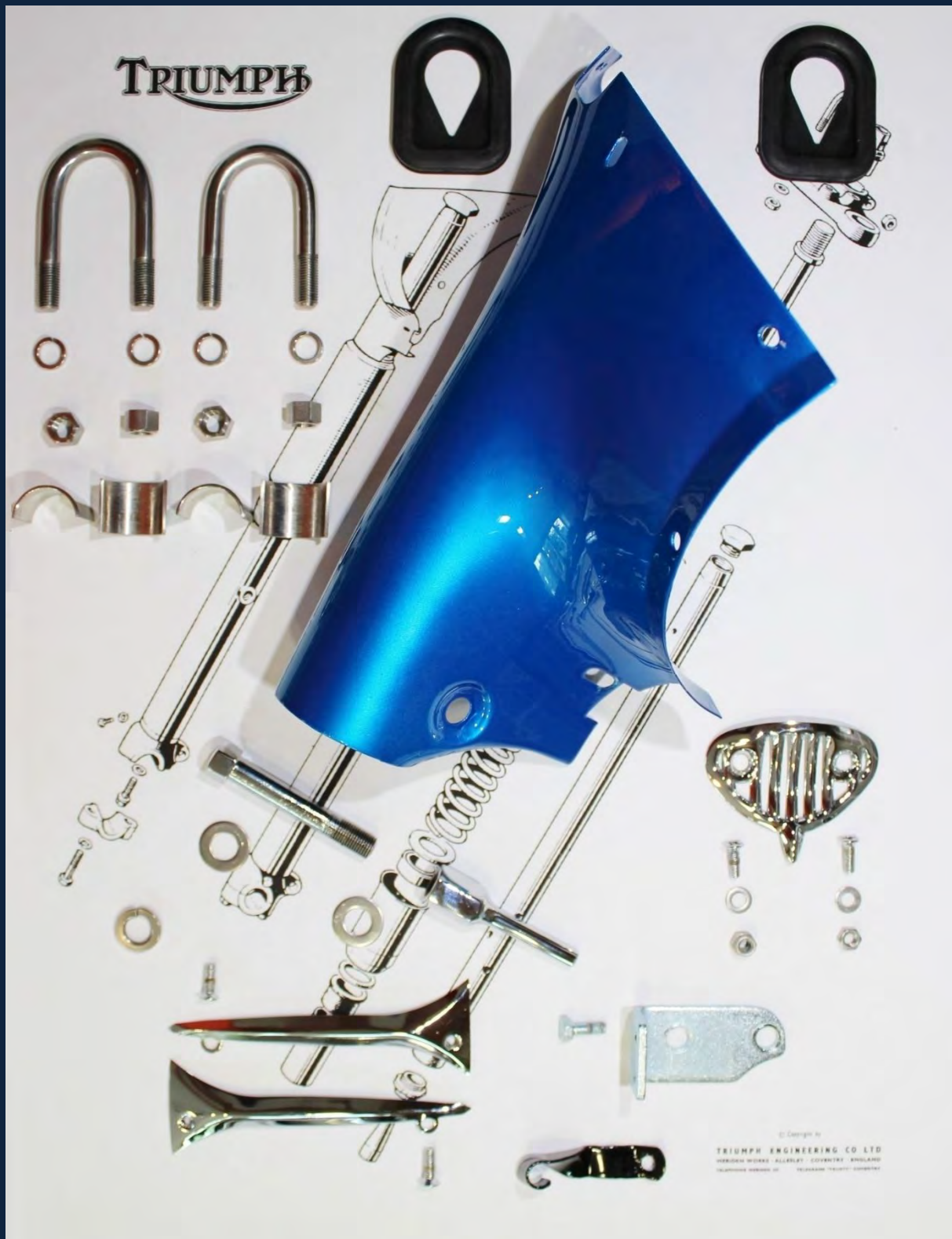
Some of the parts of the Nacelle for the 1966 3TA.
