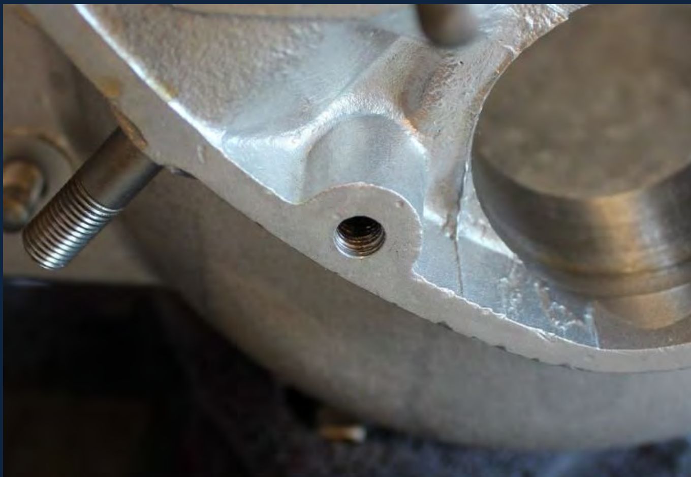
A damaged thread... a Helicoil will be needed.
