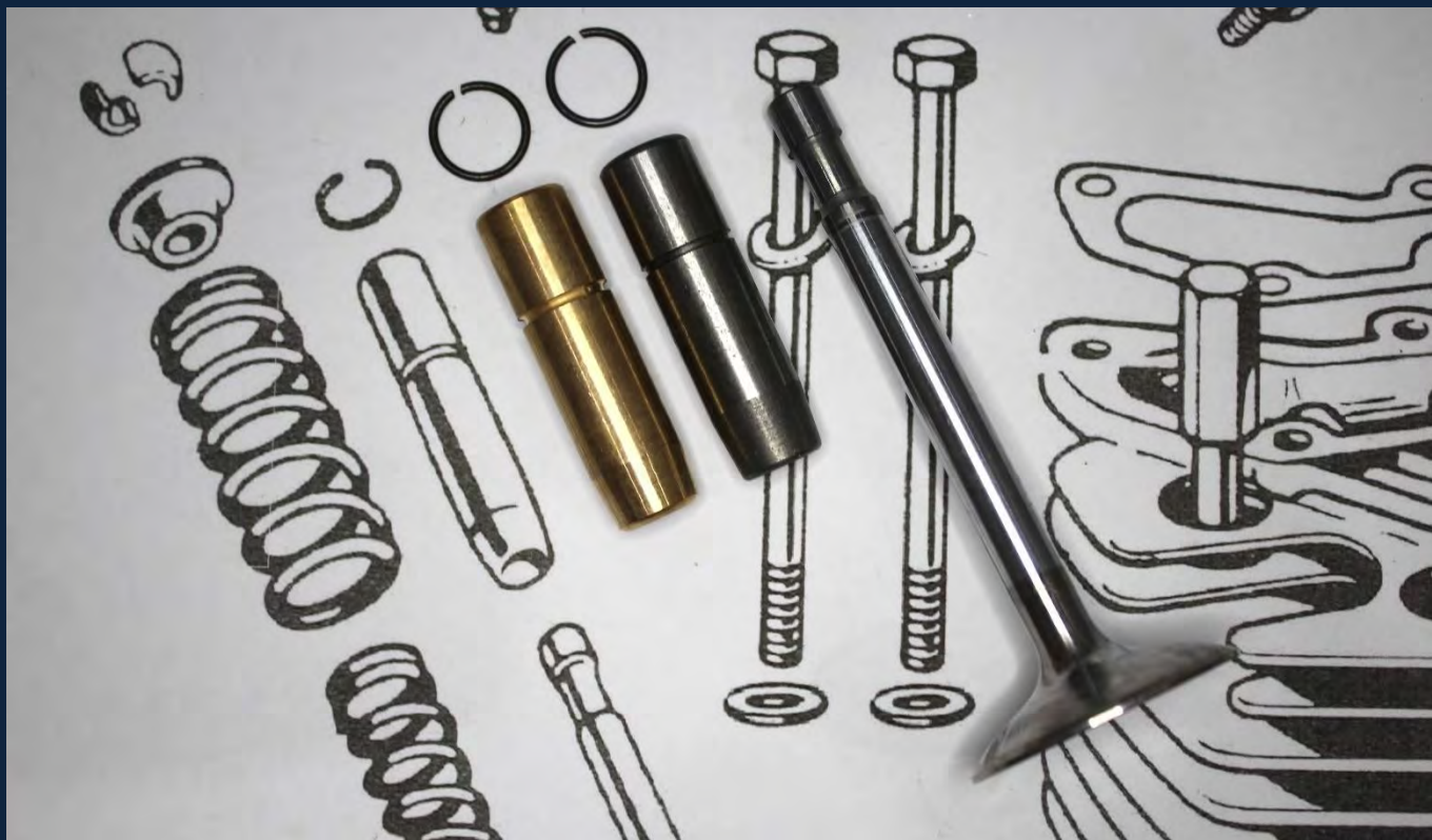
New bronze and iron valve guides and circlips.
