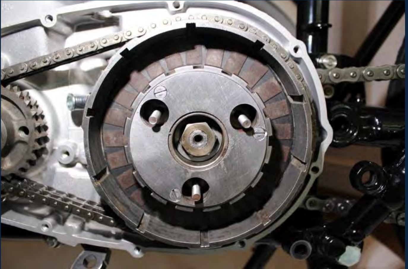
Shock Absorber and 1 st Driving Plate Fitted.
