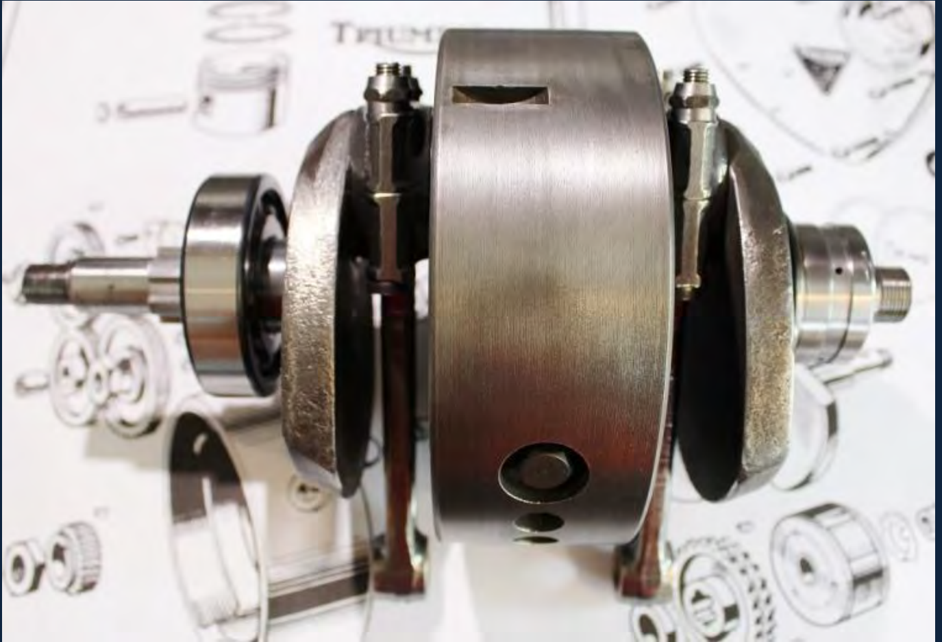
Crankshaft assembly and checking for fit.
