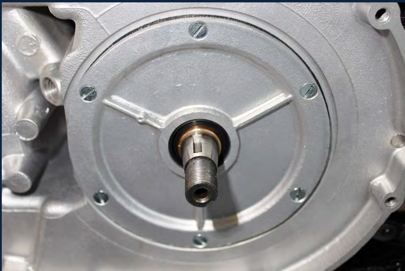
The 1966 Access Plate and the blanked off Chain Oil Feed Quill.
