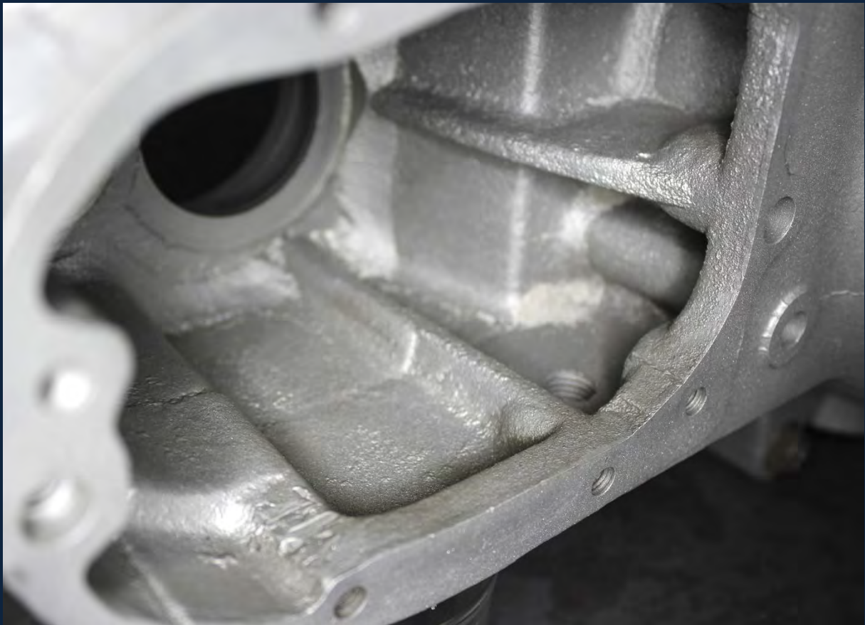
And from 1966, note the increased strength provided by the full width ribs. It is not possible to fully drain these later boxes and metallic particles or debris can collect in the recess seen here.
