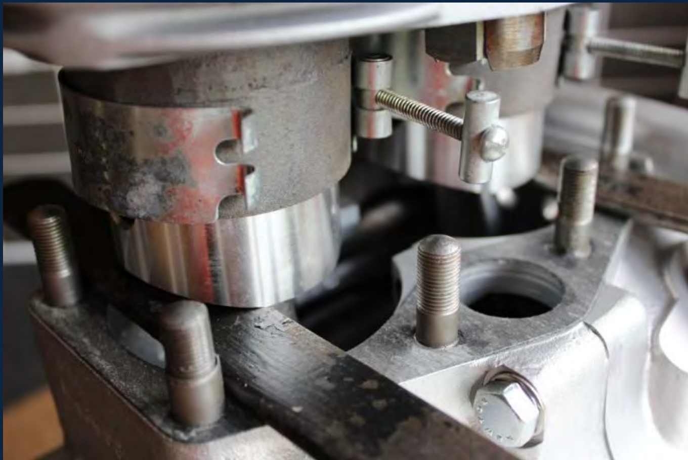
The pistons being fitted into the barrels.
