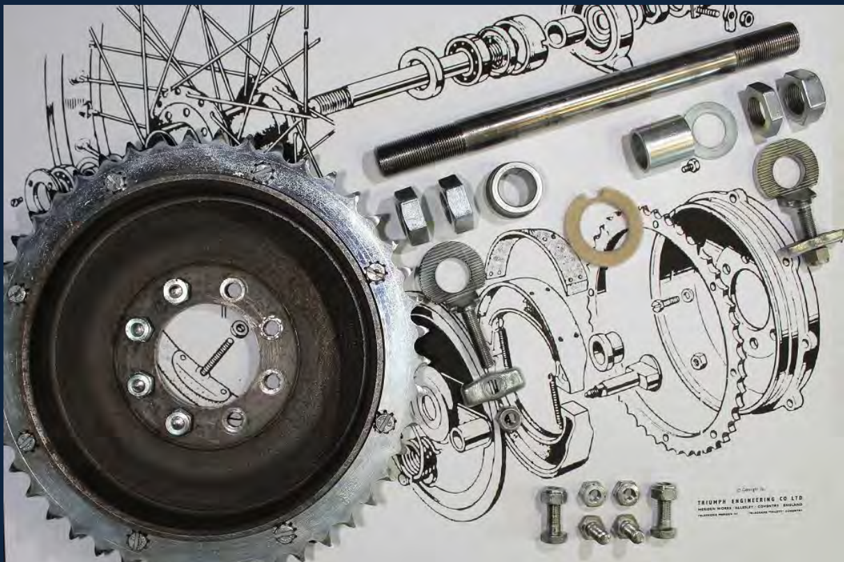
The Standard drum (non QD) and the arrangement of the axle, parts and fasteners.
