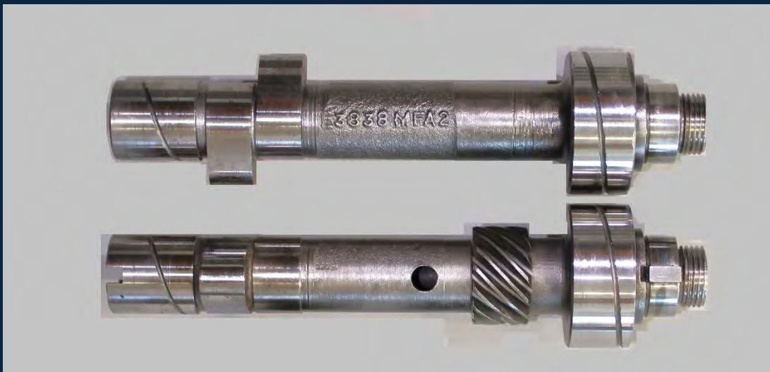
A Pair of Camshafts for the Distributor Models (to 1963).
