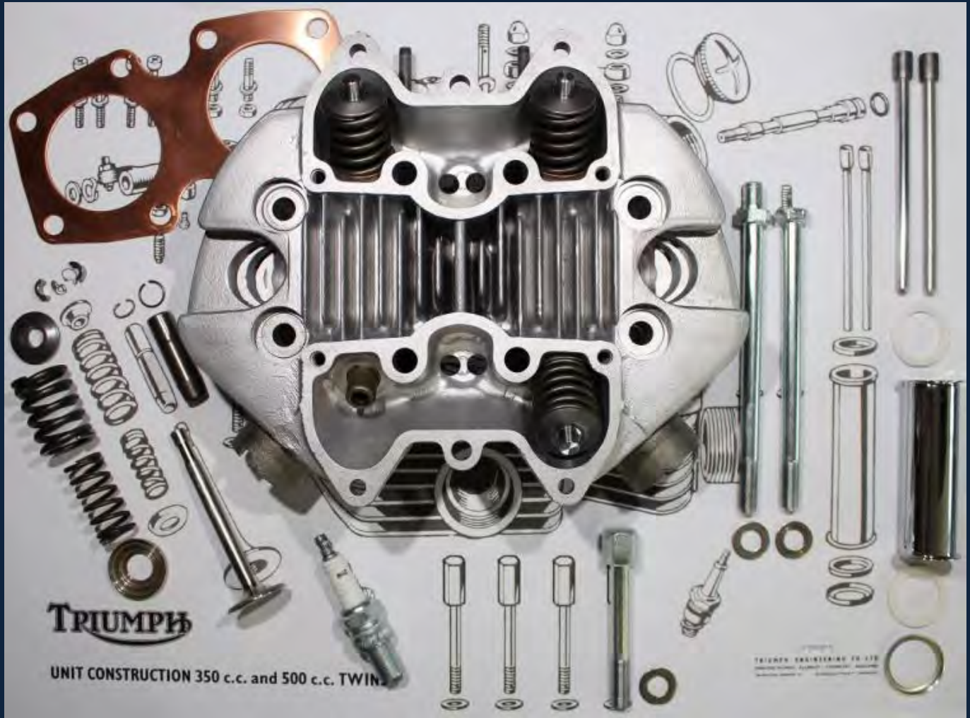
The Cylinder Head Assembly.
