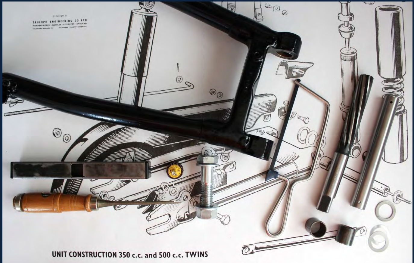
Swing Arm Spindle, Bushes, Shims and tools.
