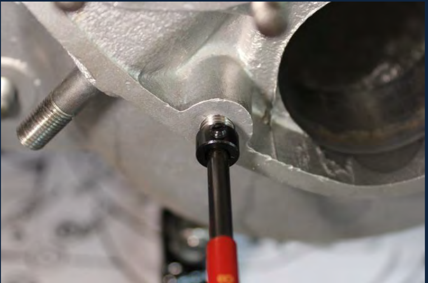
Using the supplied tool to insert the Helicoil fully.
