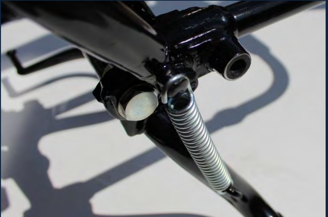
The fitted Main Stand and Spring.
