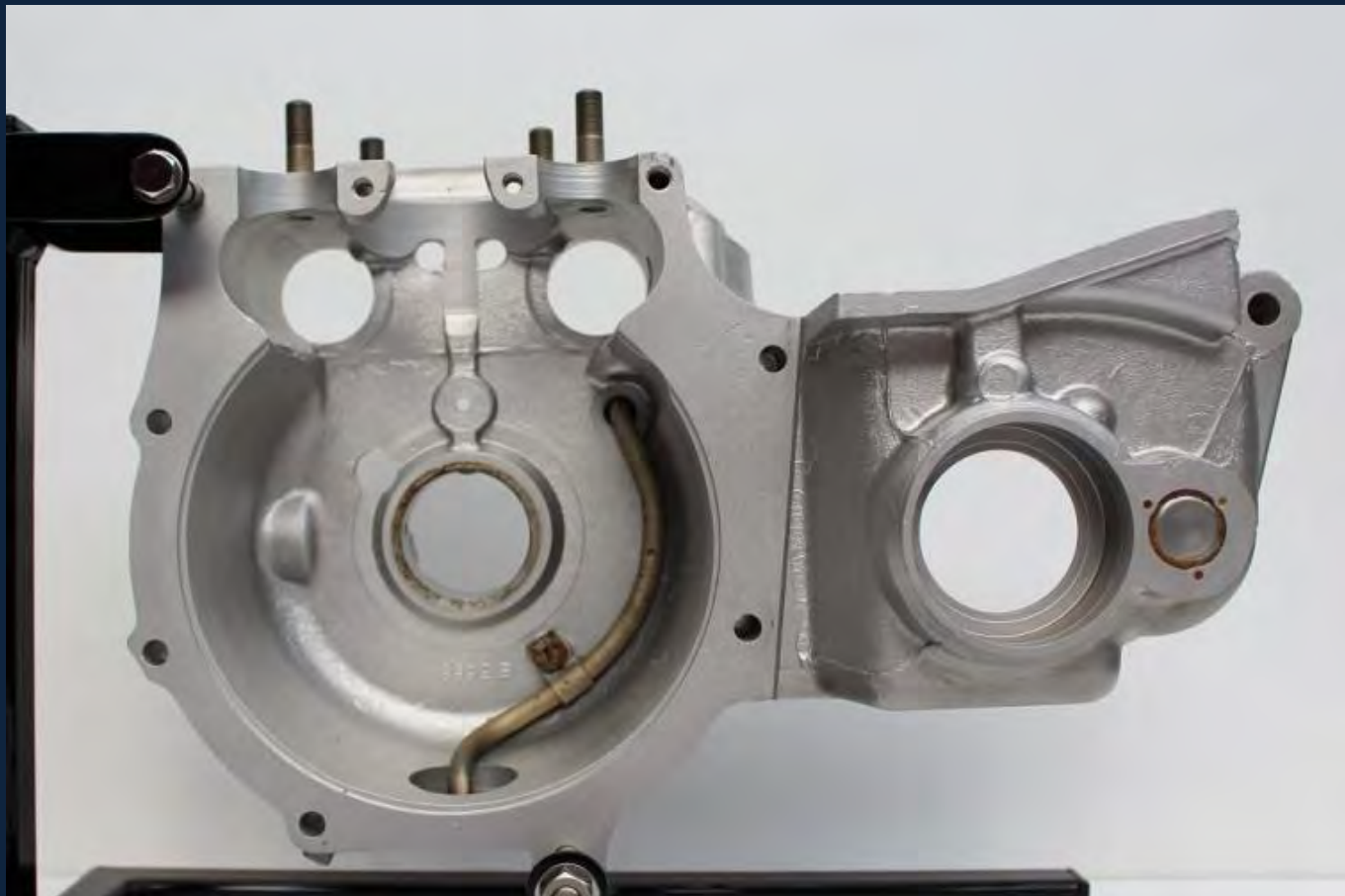
Crankcase Timing Side Internal View.
