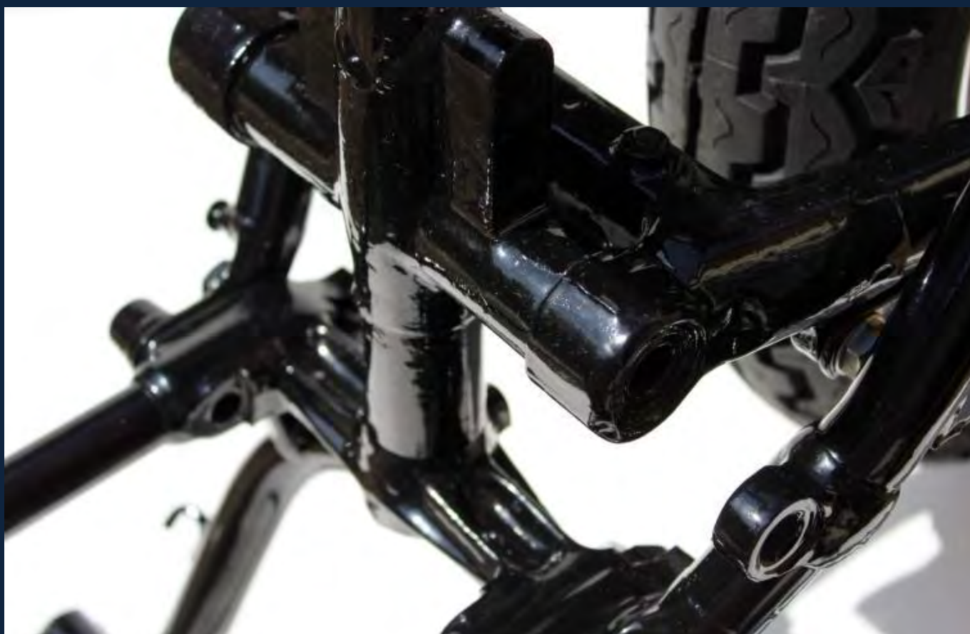
The Rear Frame and Swing Arm Pivot.
