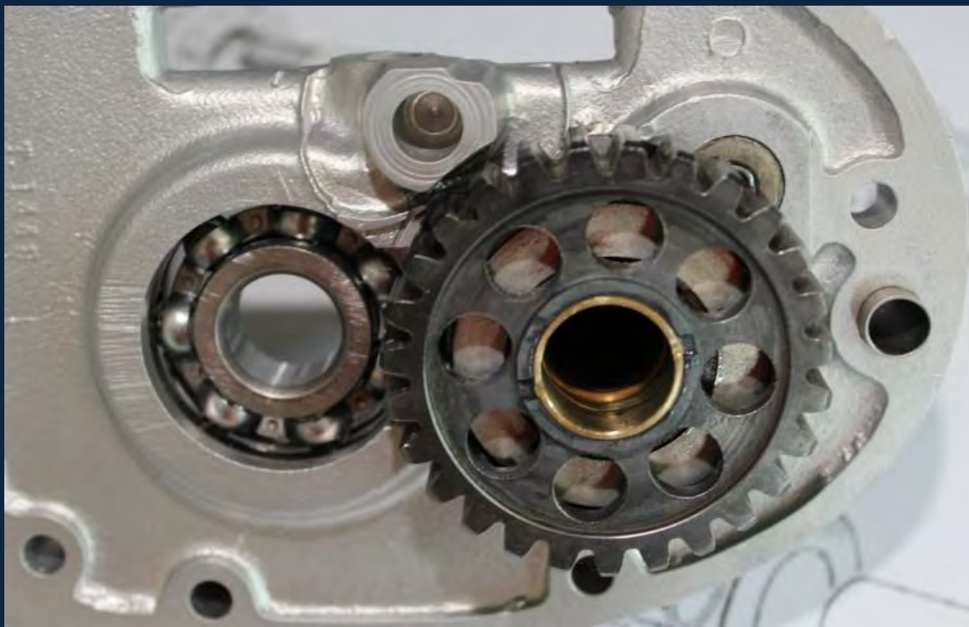
Thrust Washer and Layshaft 1 st gear fitted.
