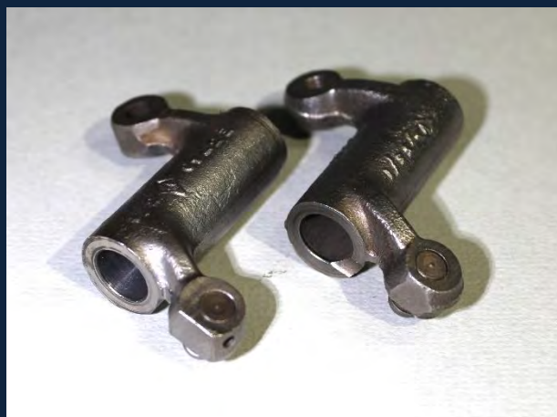
The Early (left) and Late (right) rocker, fit only matched sets. The early rocker features an oil feed to the pushrod cup.
