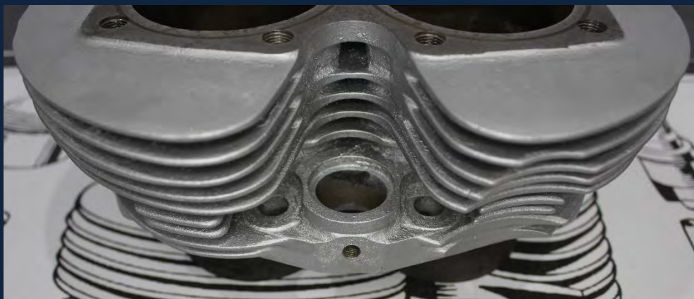
The 500cc barrels with the distinctive 'Scallop'.
