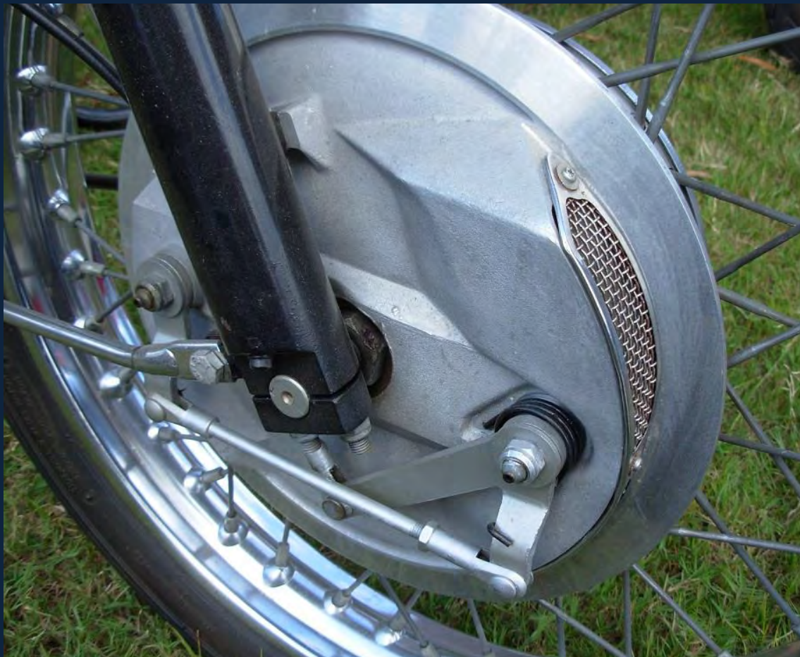
The Twin Leading Shoe Brake.
