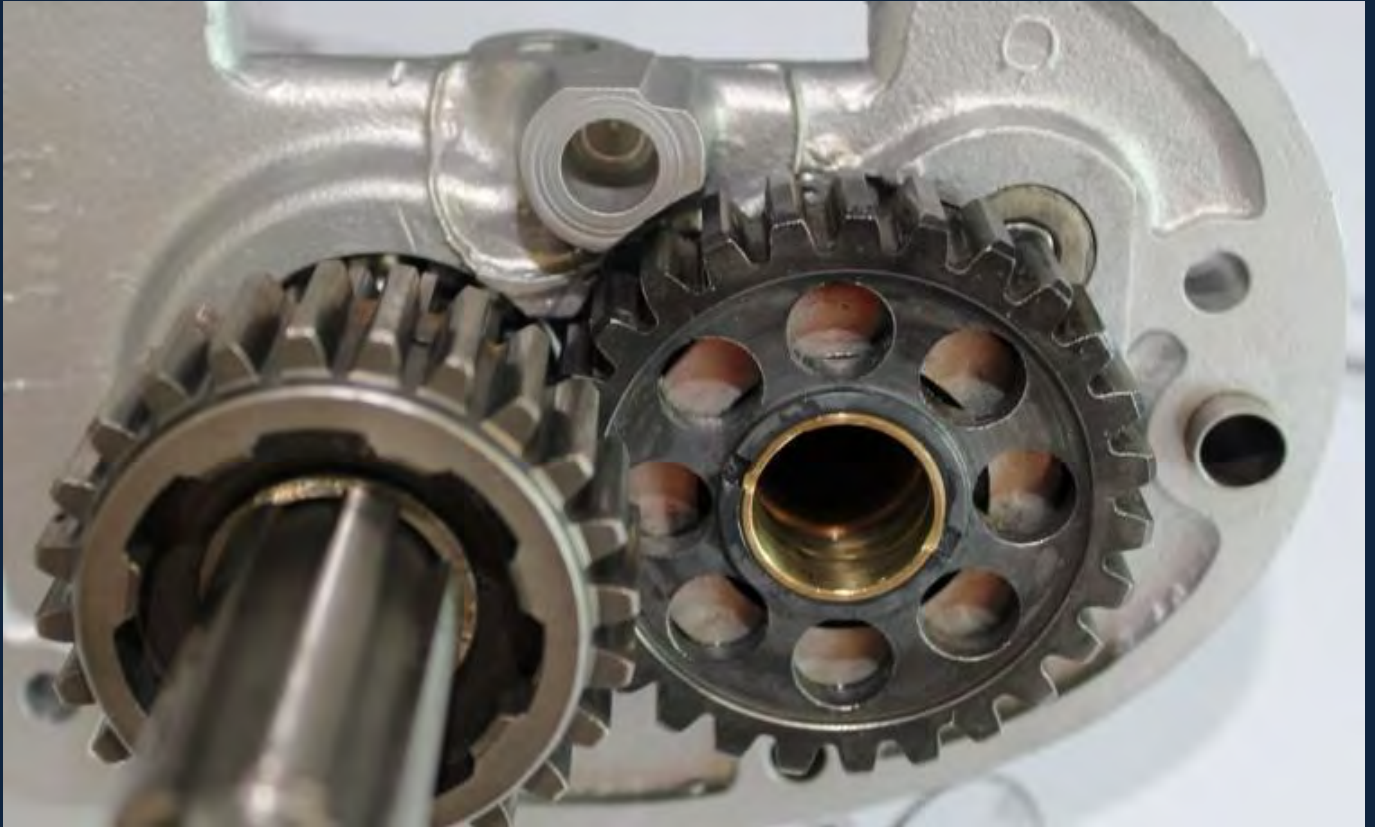
Mainshaft with First and Third Gears fitted.
