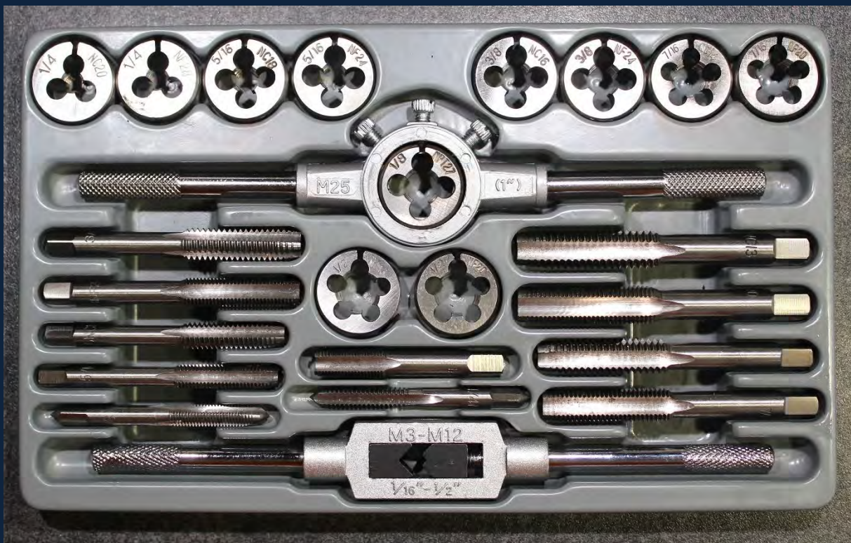
A general-purpose Tap and Die Set here in UNF and UNC.
